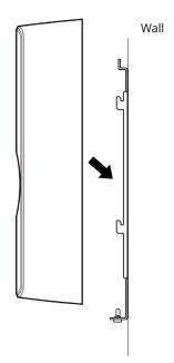
**3** Connect BioEntry R2 to the bracket by rotating the product fixing screw.
