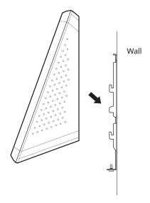
**4** Connect FaceLite to the bracket by rotating the product fixing screw of FaceLite.
