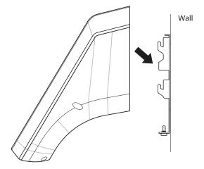
**4** Connect FaceStation 2 to the bracket by rotating the product fixing screw of FaceStation 2.
