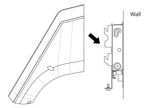
**5** Connect FaceStation 2 to the bracket by rotating the product fixing screw of FaceStation 2.
