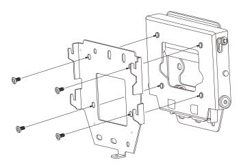
**4** Install FaceStation 2 onto the fixed bracket.
