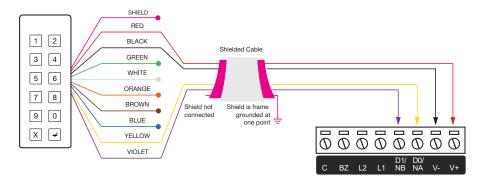
When the green and orange wires are not connected together, the reader defaults to an entry reader.
