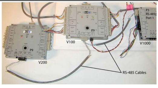
4. Interface Address – Set the interface address by turning the Address dial. Ensure that the V100 Interface Address is documented in the Hardware Installation Worksheet (found in the back of the HID VertX V1000 Quick Install guide).
